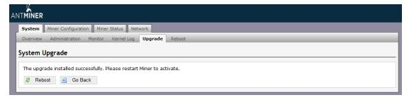
Clicking the 'Reboot' button will restart the miner so it can load the new software. Clicking 'Go Back' will keep the AntMiner mining, before switching to the new software when it is restarted next time or power cycled.
