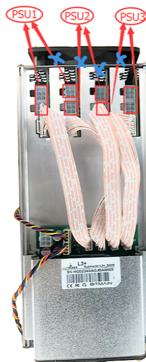
Figure 2-2. PCI-E Connectors - Incorrect Connection
