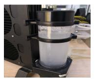
Water-cooling plates inside the server are welded parts made of aluminum, which have been cleaned before roll-out. Water in some servers may appear to be turbid after running for a period of time. Kindly note that this will not affect on the overall cooling system and long-term operation of the system.
