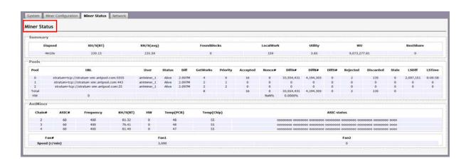
Note: The X3 server is with fixed frequency 400 MHZ. Firmware will stop running when the Temp(PCB) reaches to 80-85 °C or the Temp(chips) reaches to 125-135 °C, there will be an error message "Fatal Error: Temperature is too high!" shown in the bottom of kernel log page.
