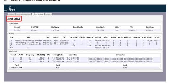
Note: The DR5 server is with fixed frequency adjustment 600 MHZ. Firmware will stop running when the Temp(chips) reaches to 100°C, there will be an error message "Fatal Error: Temperature is too high!" shown in the bottom of kernel log page.
